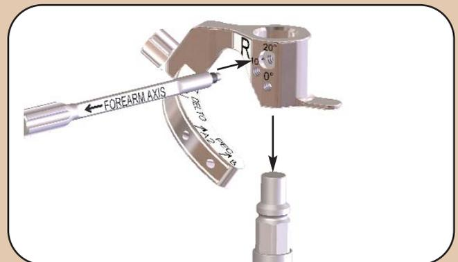
Slide the assembly onto the remaining reamer.
