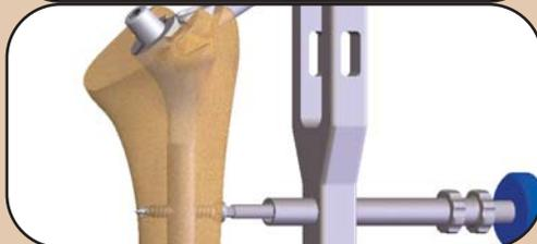
Insert the screwdriver into Ø 10 mm guide and remove the screw.
