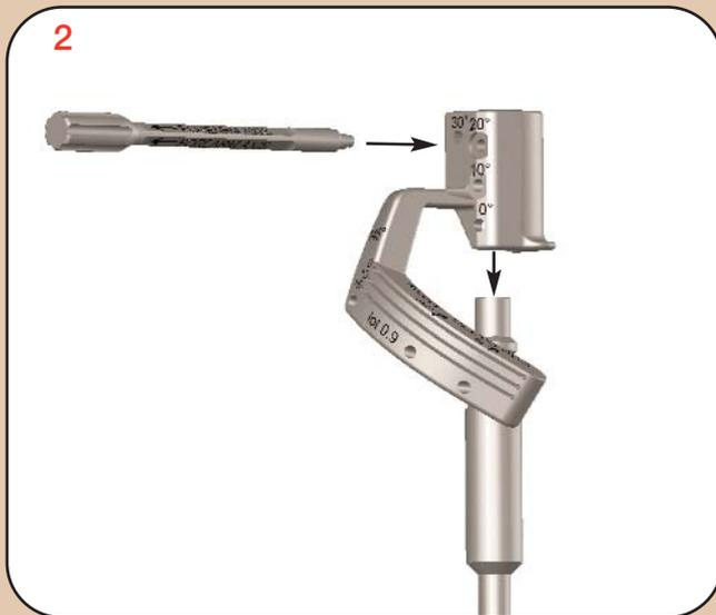
Slide the cutting guide onto the remaining reamer.
