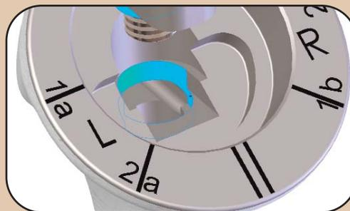
The retroversion is determined by screwing the rod into one of the 3 positions (0, 10, 20°) and aligning it with the arm. Use the Muraschowsky<sup>2</sup> criteria to set the height of the implant. When the stem position is adequate, use the benchmarks (1, 2 and 3) for the future stem impaction, and put a mark on the humerus.
