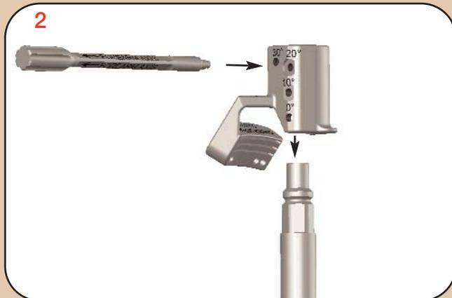
Slide the cutting guide onto the remaining reamer. Screw the retroversion stem into one of the 4 positions according to the required angle: 0°, 10°, 20°, 30°.
