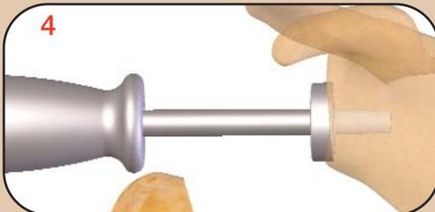
Screw the extractor into the baseplate post and remove it.
